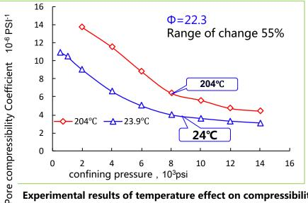
Experimental results of temperature effect on compressibility coefficient
