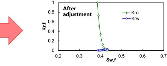
The low temperature relative permeability curve is changed, so that the production is zero under the initial temperature. The high temperature relative permeability curve keeps the same. The simulation results after adjustment are consistent with the actual thermal recovery test, which greatly improving the simulation accuracy.
