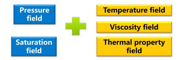
On the mechanism of Thermal recovery, thermal development needs to consider temperature field, viscosity field, thermal property field, etc. Conventional water injection development can be combined with reservoir engineering method and numerical simulation method. Due to multi-field coupling , numerical simulation has become an important predicting method in thermal recovery.
