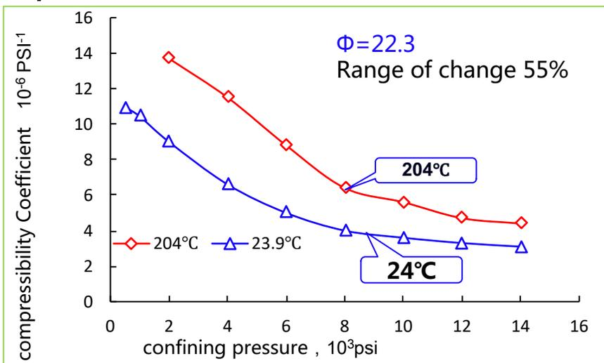
Experimental results of temperature effect on compressibility coefficient
