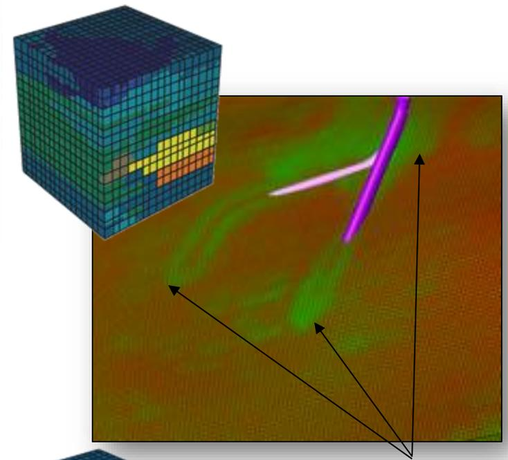
The higher resolution model successfully captured the gas condensate dropout.
