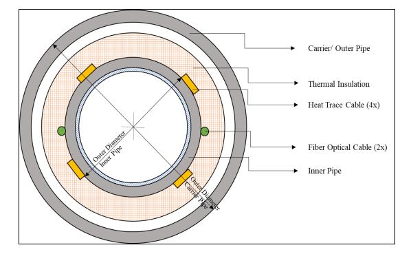
• World's longest ETH PIP as the primary layer of protection for Wax & Hydrate
