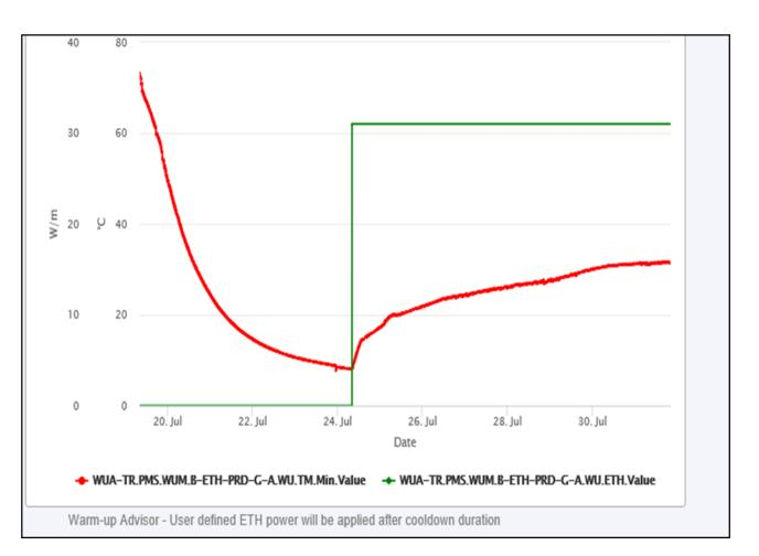
Power (green), Min Temperature in Pipeline (Red)
