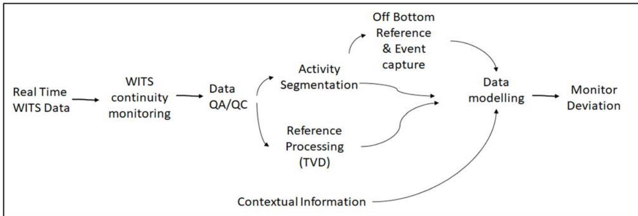
Figure 2—Data flow within the RTOC's platform
