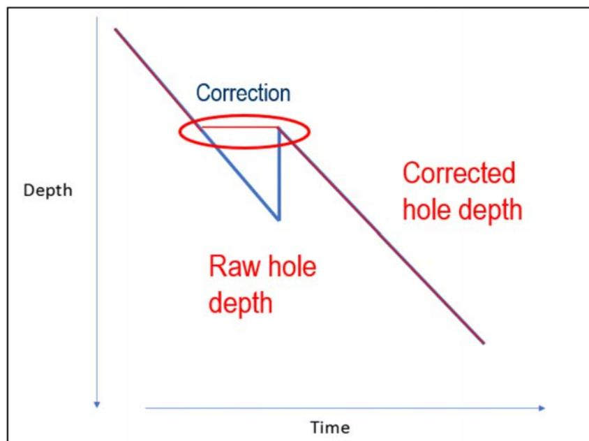
Figure 3—Example of Hole Depth Correction
