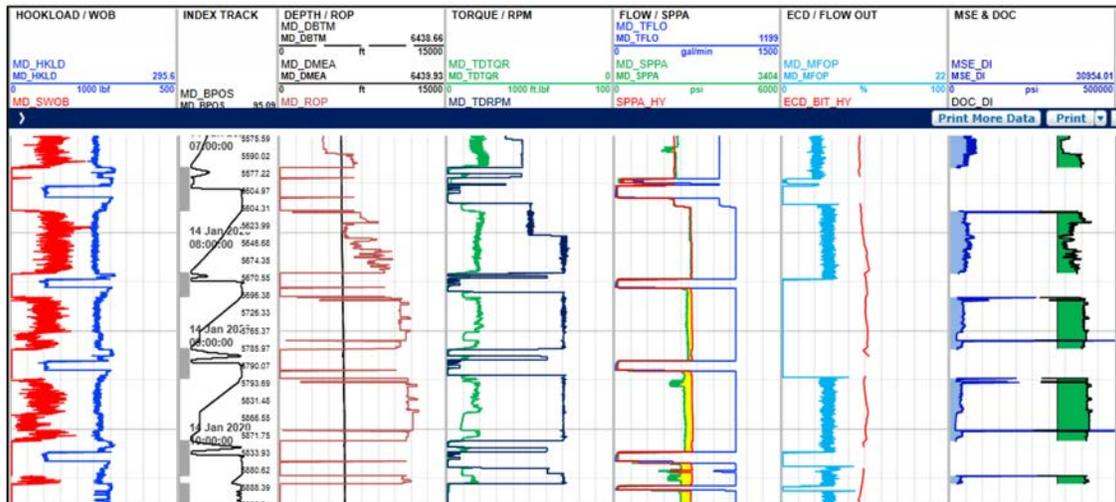
Figure 11—Modelled versus Real Standpipe pressure: Washout indication
