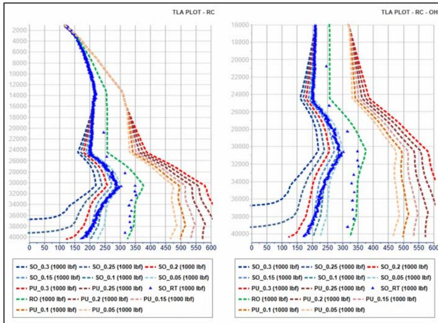
Figure 13—Broomstick versus Real Time Values for complete (left) and Open Hole section (right)
