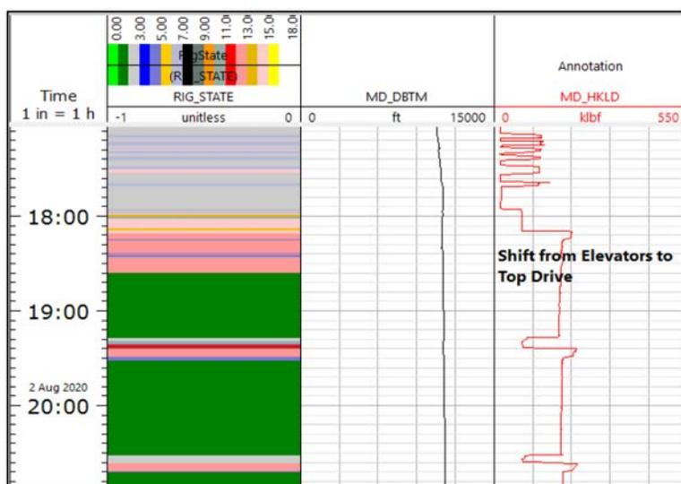
Figure 6—"InSlips" Threshold change. Elevators versus Top Drive
