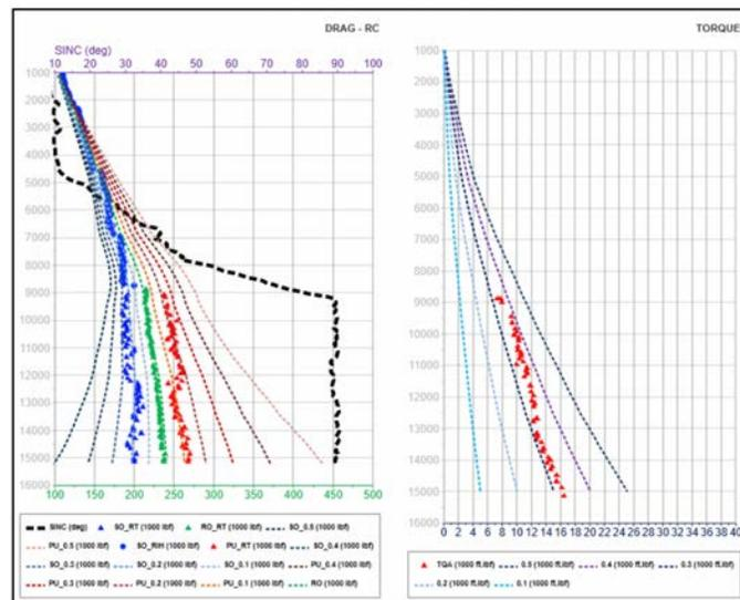
Figure 10—Torque and Drag Modelling and Monitoring
