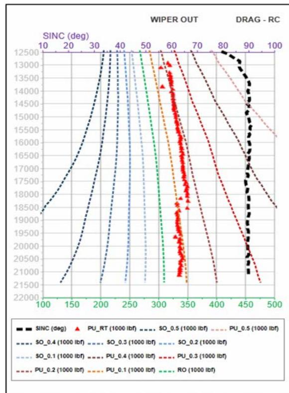
Figure 14—Drastic shift in observed "Pick Up" hookload values while tripping out with drilling BHA
