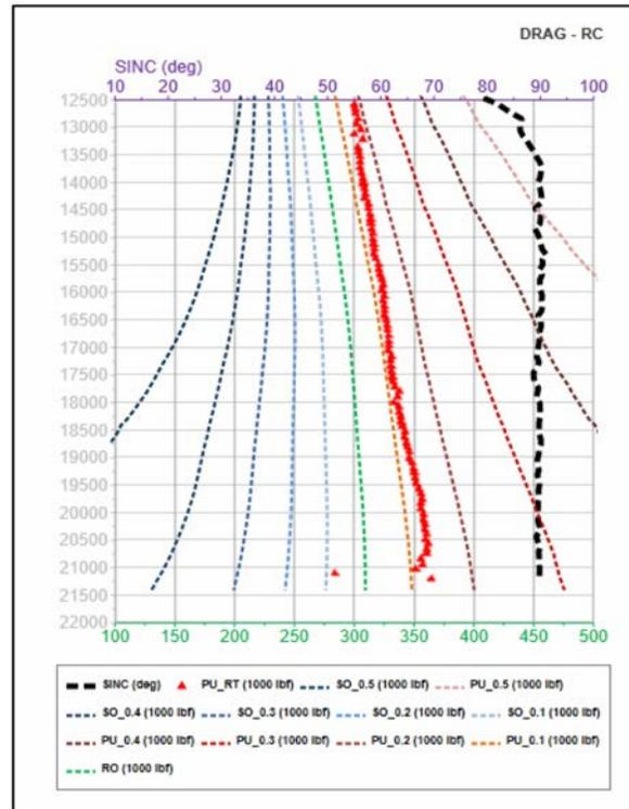
Figure 15—Pick Up Hookload values after "Wiper Trip"
