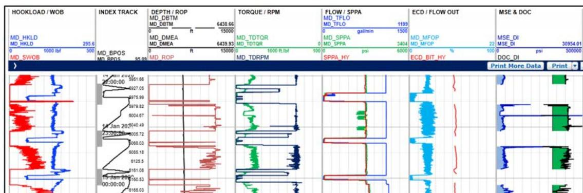
Figure 12—Modelled and Actual Standpipe Pressure during normal operations
