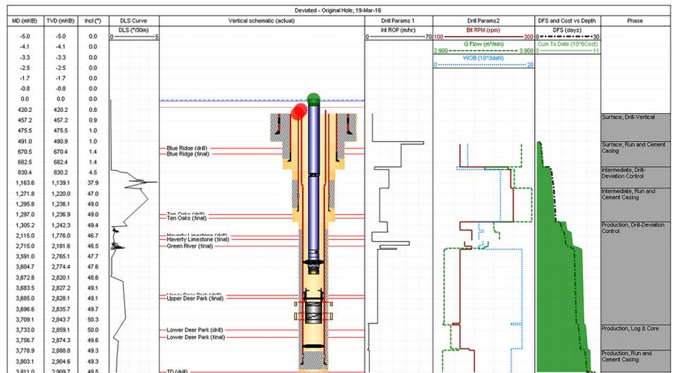
WellView’s downhole schematic is drawn from the well data to provide an accurate downhole picture at any point in time.
