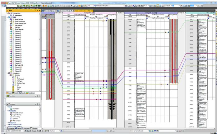
The Petrel platform's well section window brings drilling and subsurface information together, providing for clear understanding of the root causes of drilling events.
