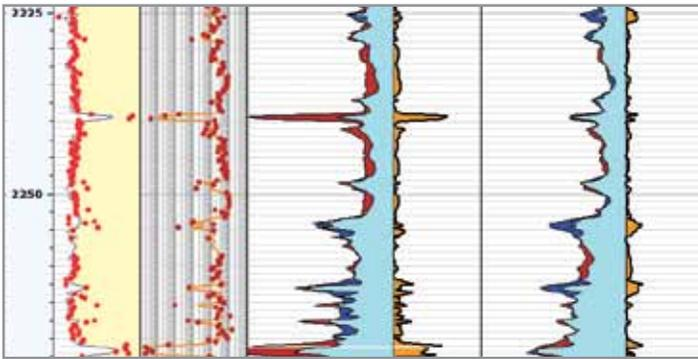
Saturation-height modeling results comparing the original core model and optimized model from the solver.
