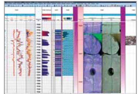
Routine and special core analysis data displayed at log scale along with core photographs in the Techlog TechCore module.
