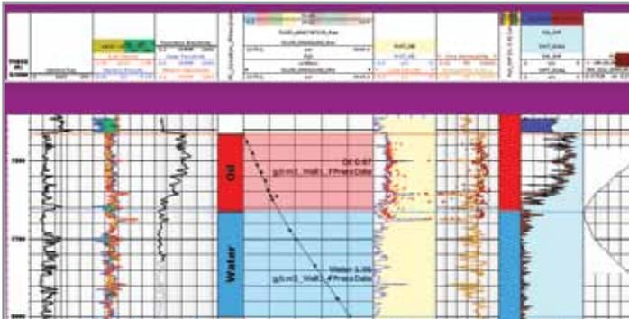
The free water level from the Saturation-Height Model module, plotted with the contact results generated in the Formation Pressure module.
