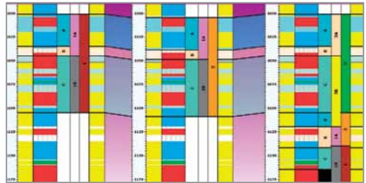
Plot showing the contacts, compartments, and fluid cores.
