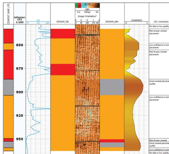
Waveform data and cement maps are used to assess probability of isolation.
