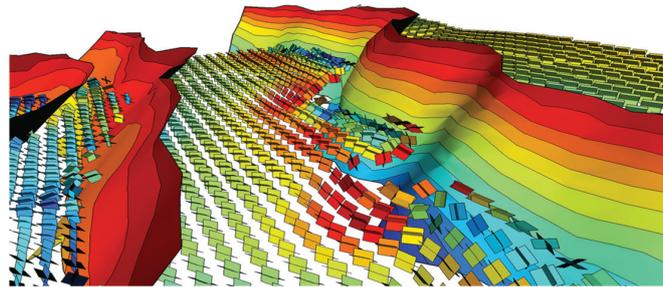
*Modeled density and orientation of subseismic faults in reservoir from Poly3D forward stress modeling.*
