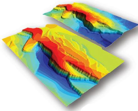
Comparison of seismic horizon (back) and Poly3D results (front) for 3D fault model QC (data courtesy of Total SA).
