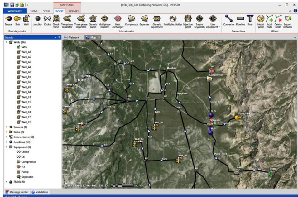
*A new GIS canvas delivers rich visual references and information to build networks. Map services can be used to augment this information—for example, a topographical map service that allows pipeline elevation profiling to be included in the model.*
