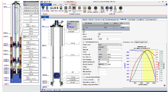
*Building wells has been made easier with a new, interactive graphical wellbore schematic shared by other Schlumberger software applications.*
