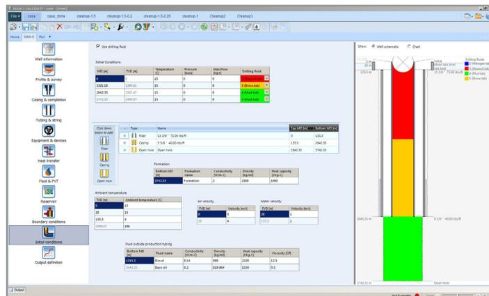
Model cleanup operations of a mud-filled well.
