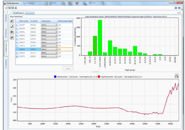
The pipeline profile generator allows large datasets to be cleaned.
