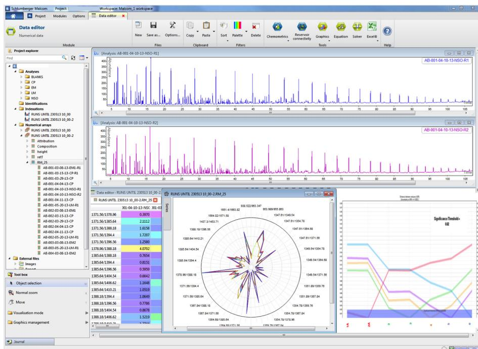
Malcom software allows comparing chromatograms for fingerprinting studies (top) as well as differentiating oil samples for quick display by using data-reduction tools (bottom center). Characterization of chemical compositional differences between oil samples (bottom right) can be performed in a matter of seconds.
