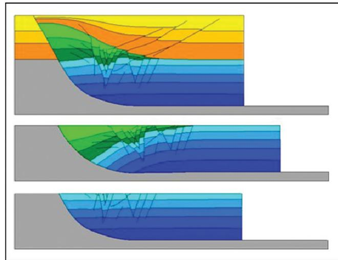
Dynel2D can restore complex inverted structures with crossing faults (sandbox model from Yamada and McClay).
