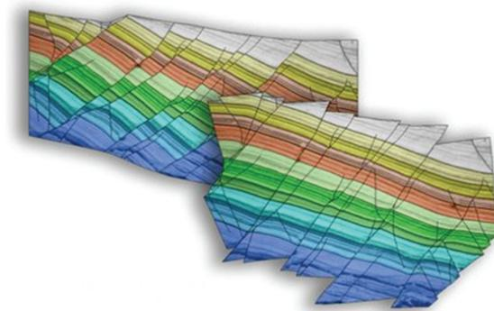
*Restored complex pattern of faults within soft sediments (data from Kristensen).*
