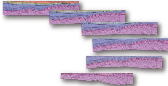
*Result from an automatic sequential restoration of a large scale basin (data from VSA).*
