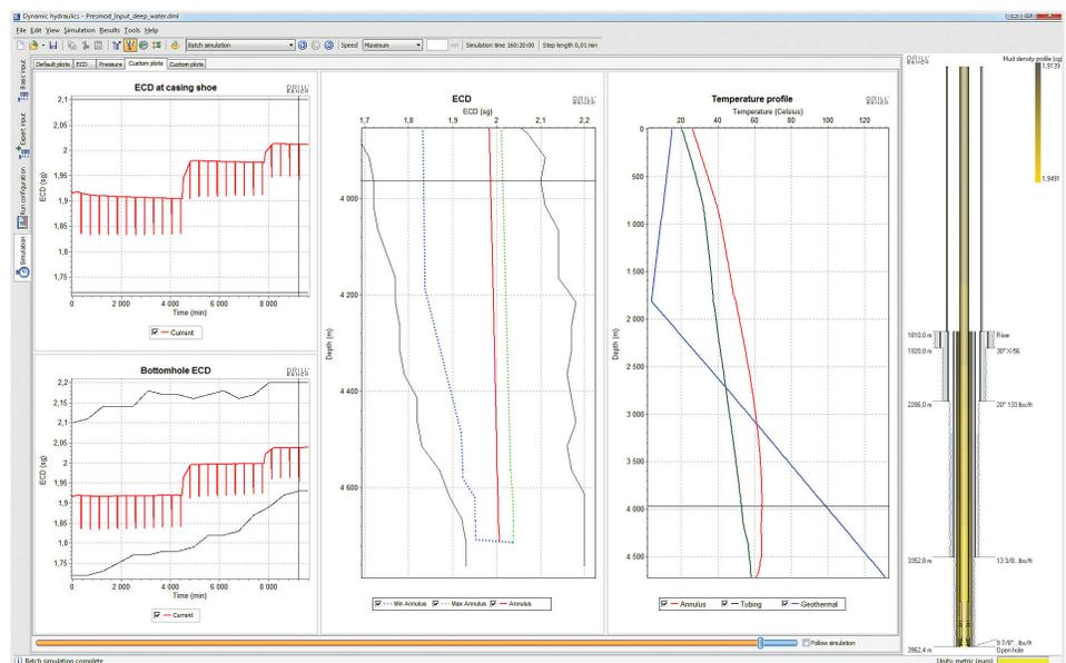
Use Drillbench Dynamic Hydraulics to model the equivalent circulating density relative to the mud-weight window when forecasting the operational pressures to ensure that the well integrity boundaries are not exceeded.
