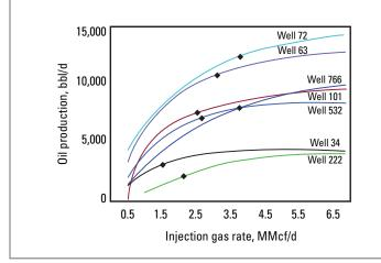
Gas-lifted wells are linked in a hydraulic model to determine the optimum injection gas rate to maximize production.
