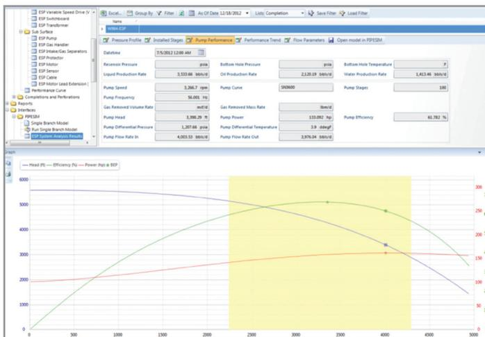
Pump operating point determination based on well performance (PIPESIM Nodal Analysis).
