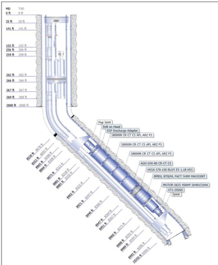
A detailed wellbore schematic allows the configuration of the equipment string, fully integrated in your production environment.
