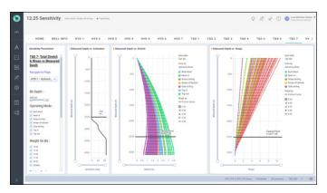
Multidimension sensitivity analysis enables you to perform multi-depth engineering analysis throughout the entire hole section. It uses interactive analytics displays with detailed engineering results for hydraulics and torque and drag in the context of your formation pressures and equipment constraints.
