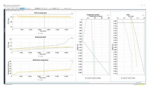
Validate that a hole section in a deep water well can be drilled with dual gradient without exceeding available drilling window.
