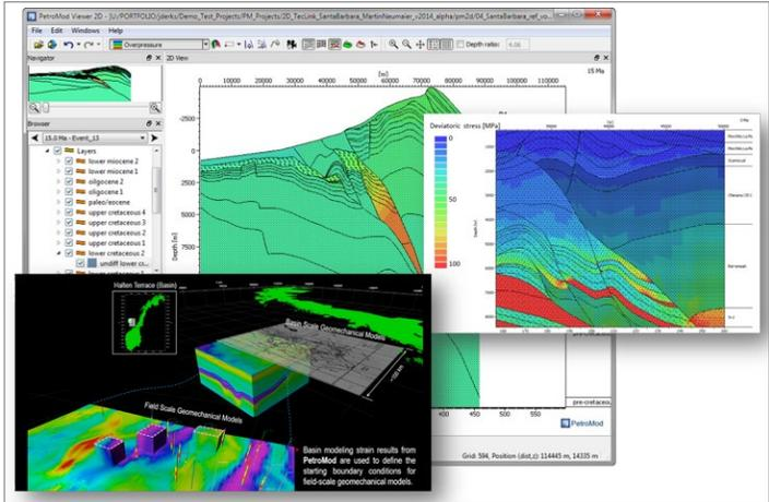
TecLink 2D and 3D in combination with the fully coupled geomechanical simulator in PetroMod software for compaction and pore pressure prediction in structurally complex areas.
