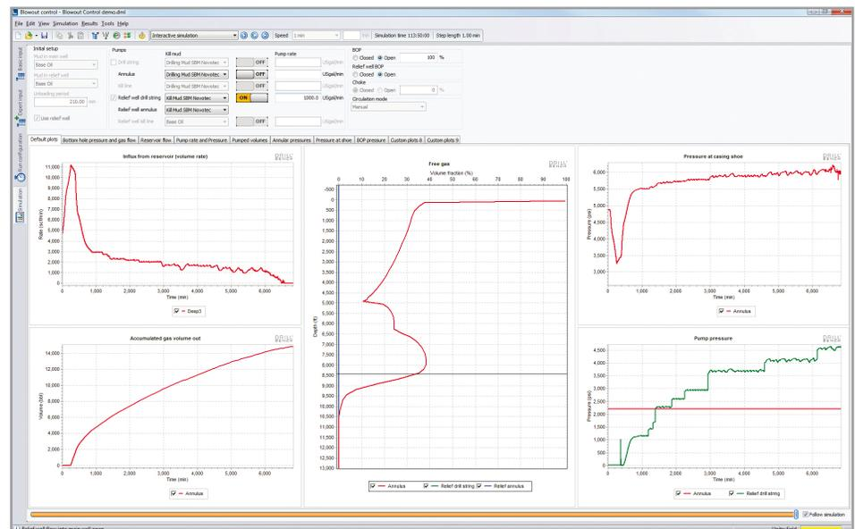
A typical blowout control simulation showing how pumping kill mud through a relief well can control and kill the blowing well.
