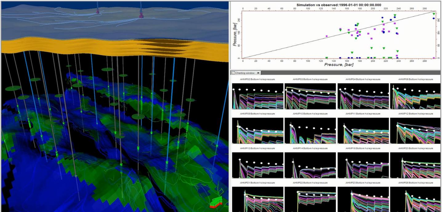
The Petrel platform enables integrated history matching studies through objective functions, a range of global optimization algorithms, and a sophisticated run management system. Extensive and flexible analysis tools are available to understand the quality of the results.
