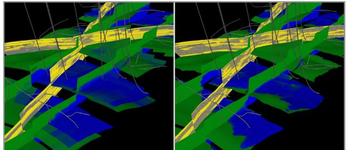
The Petrel platform offers a variety of gridding techniques, allowing models to build at appropriate scale. The INTERSECT simulator can be seamlessly used with these grids and can run geological scale models, as shown in the image on the right.
