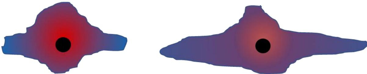
**Fig. 18—Heat map of hydraulic fractures in a gun-barrel view (red color with higher intensity represents more fracture counts and blue color shows lower fracture count). (a) More dense and shorter fracture extent with a shorter cluster spacing completion system, and (b) longer fracture length with relatively lesser density of hydraulic fractures in the near-wellbore region in a longer cluster spacing system.**
